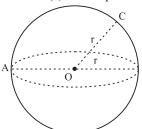
Any line segment passing through the centre and joining two points on the curved surface is called the diameter (*d*) of the sphere.
